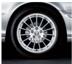
16" Antares cast alloy wheels with 205/55 HR 16 all-season tires standard on the X-TYPE 3.0 1
