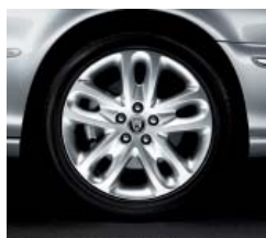
17" Aguila cast alloy wheels 4 with 225/45 HR 17 all-season tires standard on the X-TYPE Sport
