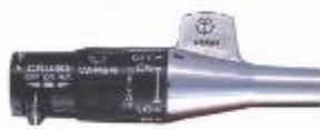
▲ The standard multi-function lever provides handy controls for intermittent wipers, washers, directional signals and high/low beam. Shown with optional electronic speed control, available only with Comfortilt steering wheel.
