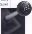
Getrag-licensed 5-speed manual transmission with overdrive. Standard with 4.3 Liter (262 Cu. In.) V6 in S-Blazer and S-10 Pickup.
