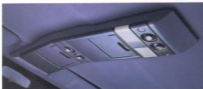
▲ Optional overhead console with sliding door compartments and four individual reading lamps.
