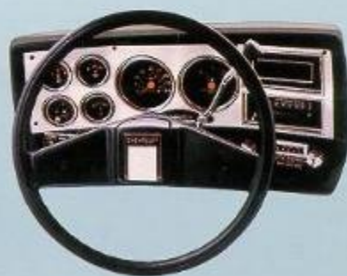
Silverado instrument cluster with standard gauge package and new trip odometer. Gauges and speedometers on Canadian-marketed Light Duty Trucks are displayed in metric units with appropriate international symbols.
