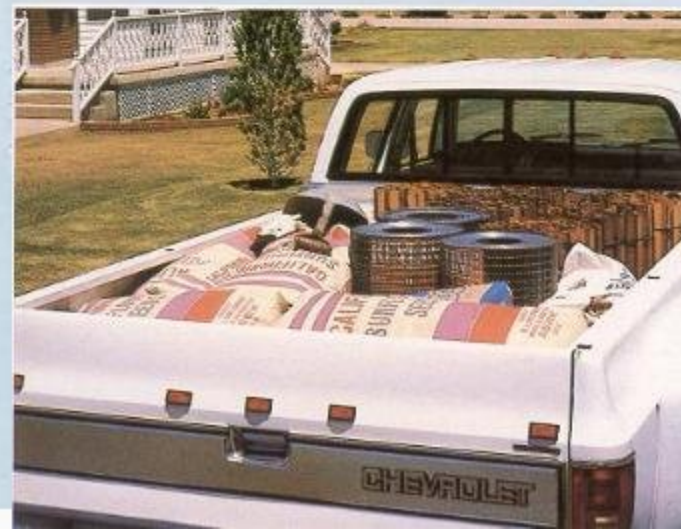
Pickups have a full-size, 2.4-m (8-ft) long Fleetside pickup box in back
