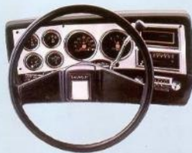
Silverado Instrument cluster with brushed pewter-tone trim and standard gauge package. Instrument cluster gauges and speedometers on Canadian-marketed Light Duty Trucks are displayed in metric units with appropriate international symbols.
