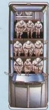
9-person seating with standard front bench seat, standard folding centre seat and available rear bench seat
