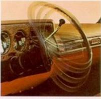
Comfortilt steering wheel adjusts to suit driver height and reach as well as seat position. Available with fourspeed manual or automatic transmis-
