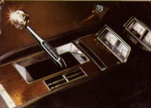
4-Speed transmission with a Hurst shifter and Special Instrumentation on console.
