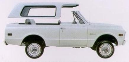
TOP-ON, TOP-OFF VERSATILITY—Weathertight reinforced fiber glass hard top bolts to the Blazer and is easily removable. Includes windows and ventipanes for side doors.
