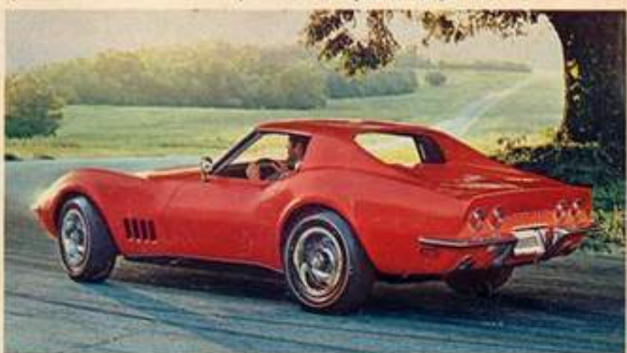
Below: Corvette Sting Ray Sport Coupe has removable rear window and roof sections. Air spoilers — front and rear — are part of its aerodynamic design.
