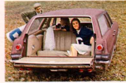
Wide third seat for 9-passenger wagons faces aft... converts to cargo area easily.
