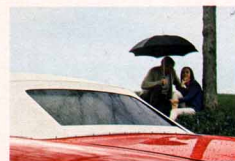
Rear window of Impala and Impala Super Sport Convertibles is tempered plate glass.
