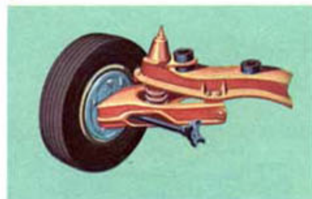
Four-point mounting of rear suspension unit is completely rubber cushioned for maximum protection against shocks and bumps.
