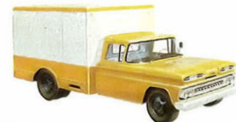
CHASSIS-CAB MODEL C3603 with special van body—With 10,000-lb. maximum GVW, you can pack in extra pounds of payload. Chevy chassis-cabs are ideal for nearly all special bodies.
