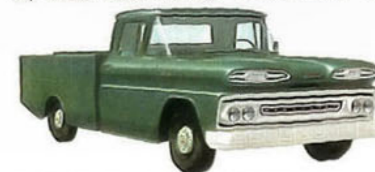
CHASSIS-CAB MODEL C1403 —Special utility body mounted on a 115" wheelbase chassis-cab demonstrates versatility; and 5,200-lb. maximum GVW allows for plenty of heavy equipment.
