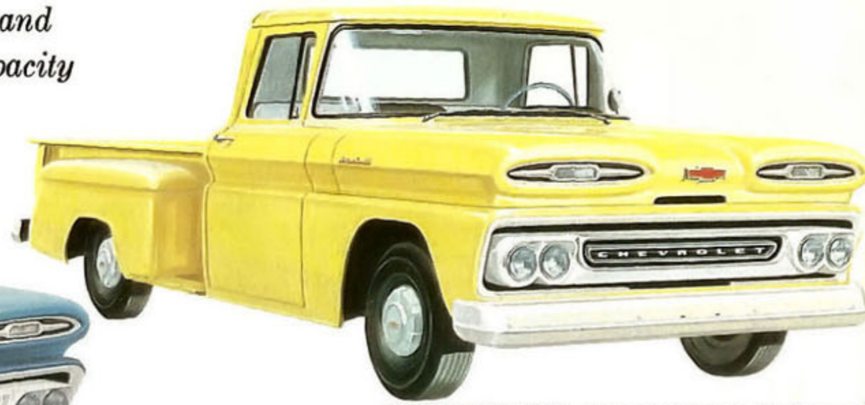
STEPSIDE MODEL C1404 —Here's a handy hauler with select-wood floor and grain-tight tailgate. Running boards make side loading a snap. High 5,200-lb. maximum GVW with an unobstructed floor area 78" long and 50" wide. Stepside models C1504 and C2504 feature a 98" box for bigger loads.
