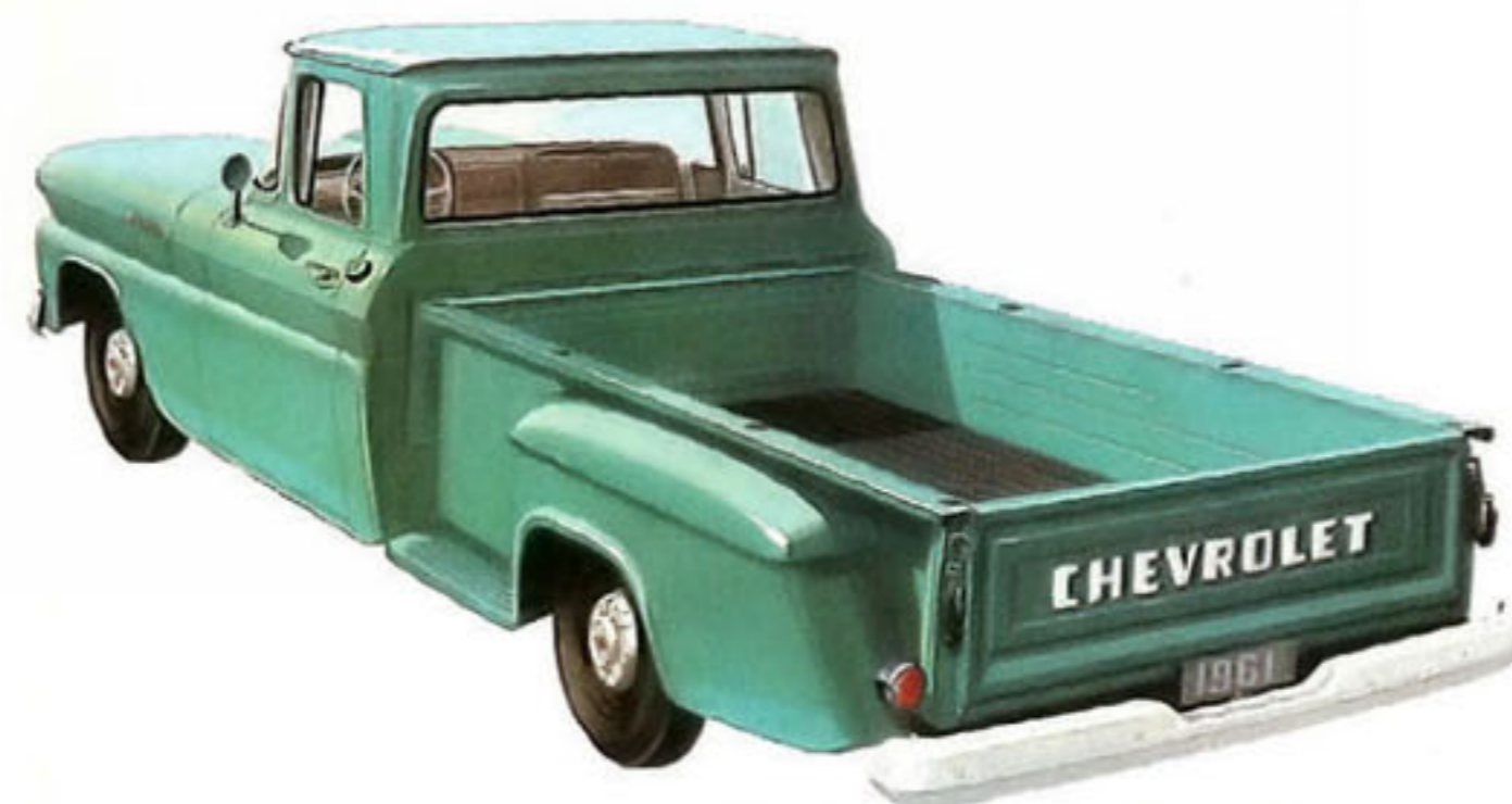
STEPSIDE MODEL C3604 —This is a big one, with a maximum GVW of 7,800 lbs. Big-capacity pickup box is a full 108" long and 50" wide for hauling out-sized loads. Powered by the standard Thriftmaster 6 or Trademaster V8 (optional, extra cost).
