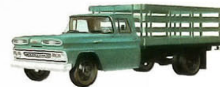
STAKE MODEL C4309 —For farm, factory and many other specialized jobs, Chevrolet offers rugged 8-, 9- and 12-ft. hardwood stake bodies with maximum GVW's up to 14,000 lbs.
