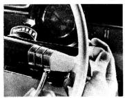
may be moved to "Low" where it will, without the slightest hesitation, throw the complete braking power of the engine into action. This should not, of course, be done except in emergencies, but IF you need it, you HAVE it in a Chevrolet!
