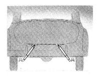
BALANCED RIDE. To further increase the stability and balance of the new Chevrolet, diagonally placed, airplane-type shock absorbers offset any tendency of the car to sway or rock on curves or when passing large vehicles at high speed.
