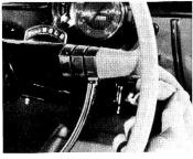
especially when road traction is lacking, the gentle, rocking-motion gained by moving the car from "Low" to "Reverse" and back to "Low." frees the car with only a minimum amount of effort on the part of the driver.
