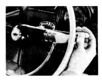
simplified controls. With the control lever in "Drive" position, the new Chevrolet with POWER-glide is ready for all straight-ahead, "stop and go" driving. This frees the driver to concentrate his attention on road and traffic conditions, since he has only to steer the car and apply the brakes or step on the gas as needed. Chev-
