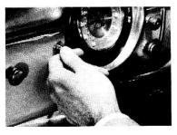
POSITIVE STARTING. With the control lever in "Neutral," Chevrolet's push-button starter goes into mesh with the flywheel before the motor begins to turn. The gear stays engaged until the starter button is released. This exclusive Chevrolet feature insures quick, easy, positive starting.
