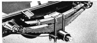
Auxiliary Rear Springs. Available for Series 4000 models. Std. on 5000, 6100, 6400. Combined Cap. 7000 lbs., each.
