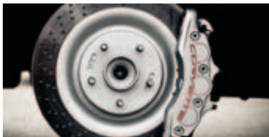
Silver calipers 1 shown with larger cross-drilled brake rotors for 427 Convertible, Z06 and Grand Sport.
