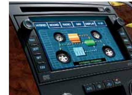
Power flow diagram on the navigation radio screen lets you see how the hybrid system is currently functioning.
