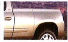
The bed is accessible by two side-access doors positioned directly behind the cab, in addition to a traditional tailgate.
