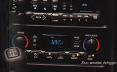
Electronic temperature control and dual-zone (driver/passenger) climate controls are optional.
