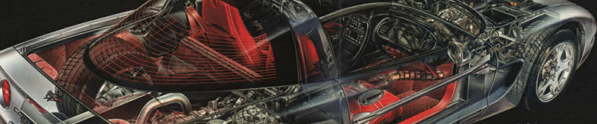
Convette features composite outer body panels that will never rust. The door outer. panels, fenders and rear quarter panels are made of flexible composite material. which protects against minor dents and dings.
