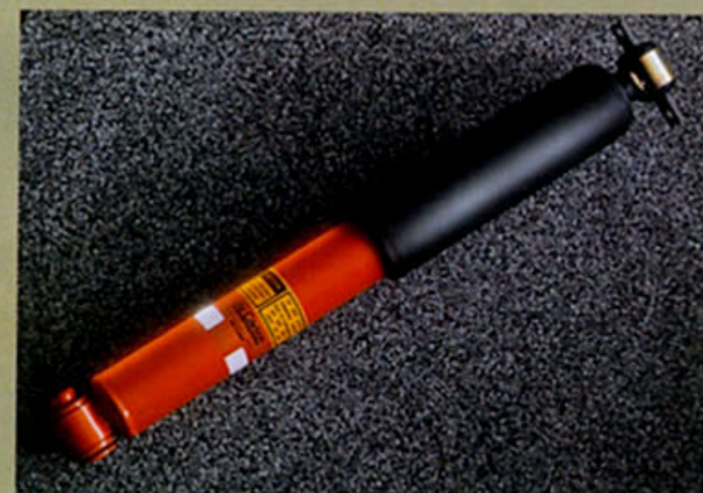
A specially-tuned de Carbon shock absorber and coil spring at each wheel deliver impressive ride characteristics while maintaining road feel. The special Ride and Handling Suspension also includes tuned front and rear stabilizer bars.
