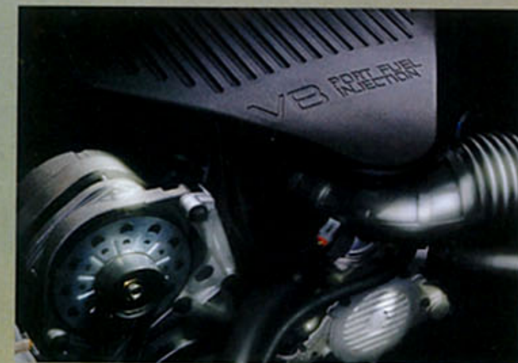
The 5.7 Liter V8 with Sequential-Port Fuel Injection delivers 260 horsepower at 4800 rpm. Platinum-tipped spark plugs are designed to last up to 100,000 miles.
