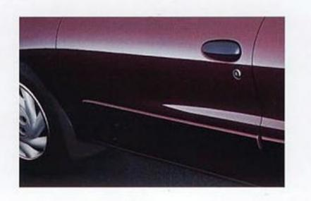
Two-side-galvanized steel is used for all body panels except the roof (where it is not needed). With this type of steel, minor scratches and chips actually "seal" themselves over time, reducing the chance of damaging surface rust developing. This is protection against corrosion that is unsurpassed in the auto industry.
