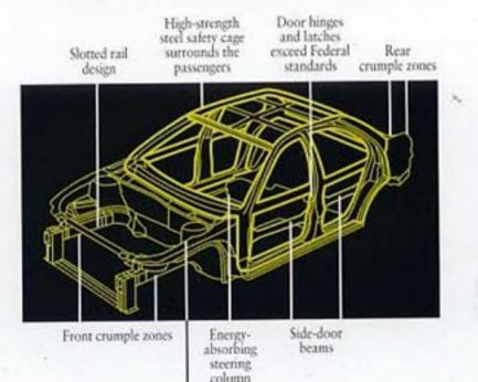
Cross-car beams for side impact Energy Absorber. Cavalier features an innovative slotted-rail chassis design that helps absorb energy in a frontal collision.
