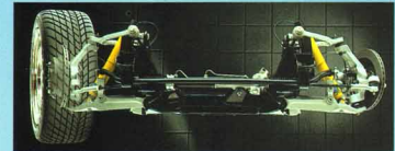
RACING-INSPIRED FRONT SUSPENSION The Corvette front suspension features high-strength forged-aluminum componentry and quick-ratio power rack-and-pinion steering.
