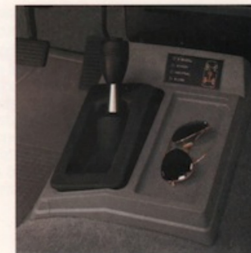
Insta-Trac transfer case provides shift-on-the-fly convenience.
