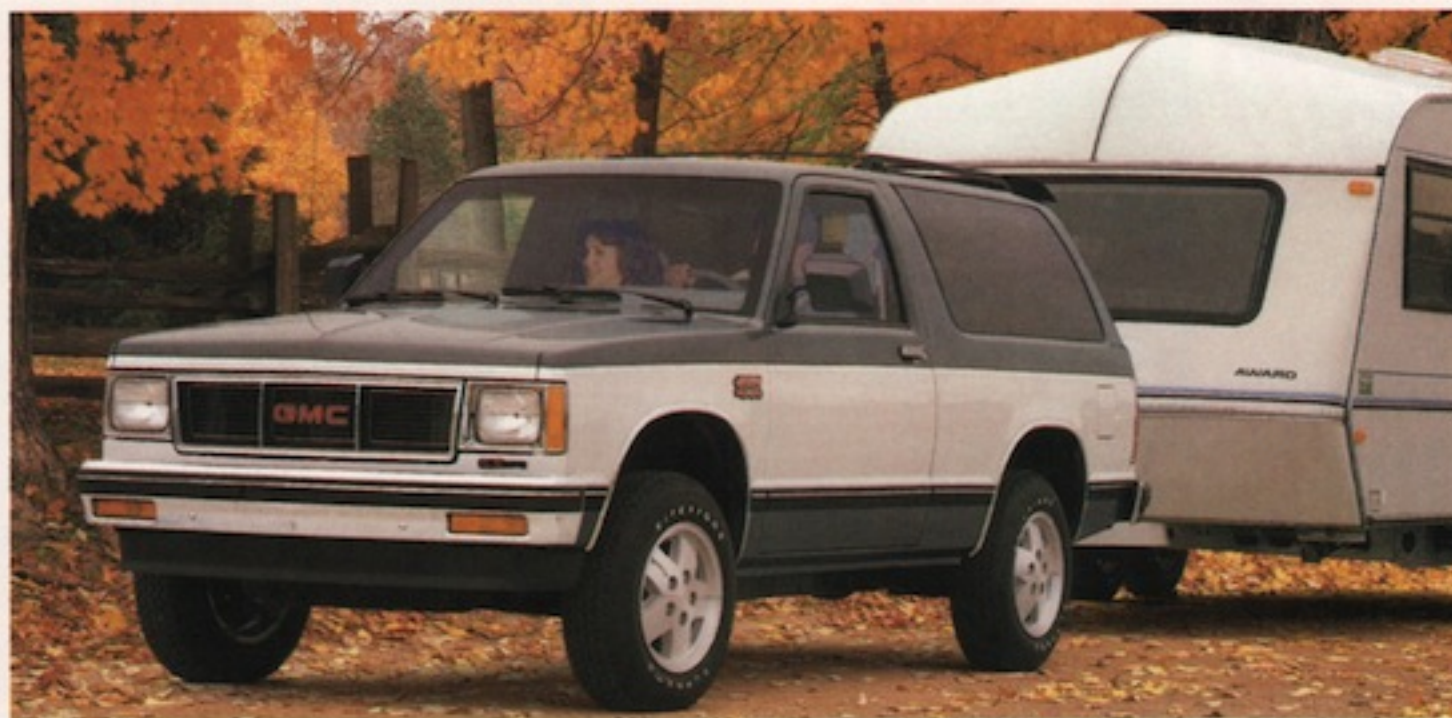
Properly equipped, 4-WD S-15 Jimmy can tow gross trailer weights up to 5500 lb.
