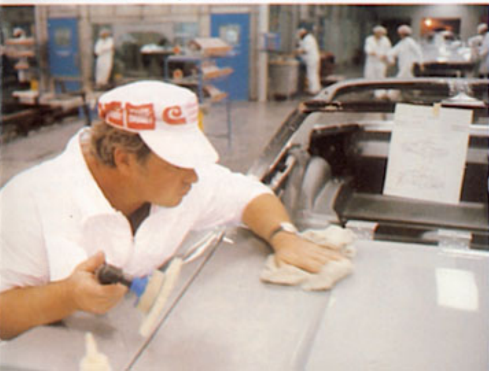
After a final clear coat, the finish is hand-polished and imperfections noted and removed.
