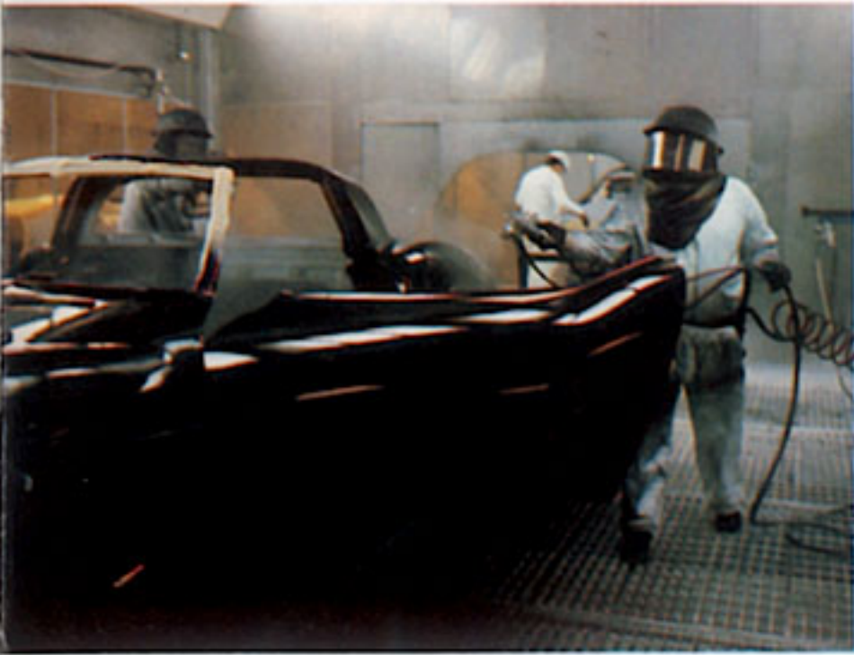
Worker applies base coat in a virtually dust-free, special paint section of the line.
