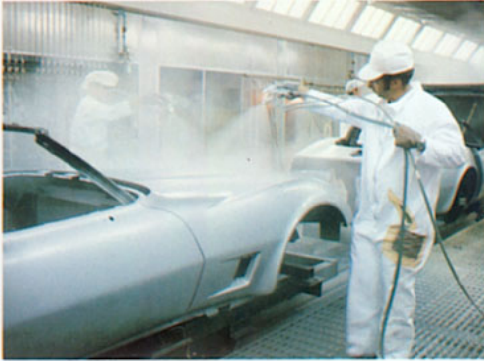
The first of six coats of color is applied to the body by spray gun specialists.
