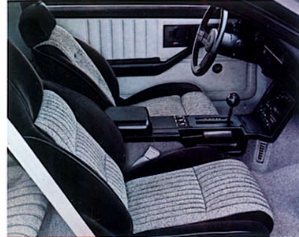
Above: Z28's new optional L/S Contour driver's seat. Left: Z28's instrumentation includes tachometer, trip odometer, voltmeter, temperature and oil pressure gages.
