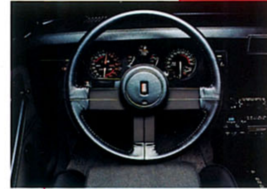
Above: Z28's new optional L/S Contour driver's seat. Left: Z28's instrumentation includes tachometer, trip odometer, voltmeter, temperature and oil pressure gages.
