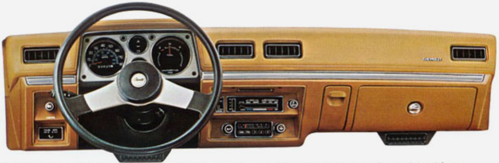
Standard color-keyed instrument panel* shown with available intermittent windshield wiper system, electric rear window defogger control, air conditioning and AM/FM radio.
