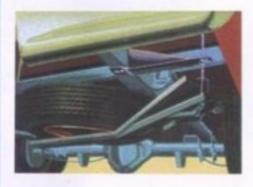
Swing Away Tire Carrier Allows extra space inside vehicle; also swings away from traffic to facilitate tire changing.
