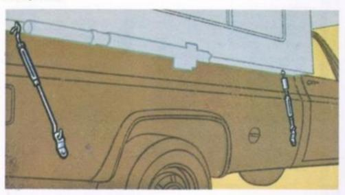
Shock Absorber Package Increases high wind stability when traveling at higher speeds or in gusty winds. Helps eliminate jerky camper motion.
