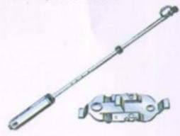
Front Bumper Tire Carrier Heavy steel brackets hold spare tire and wheel in handy position for quick easy use.
