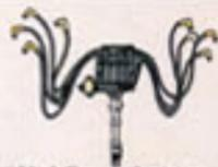
\*High Energy Ignition (HEI) produces up to 85% hotter spark for quick starts. No points or ignition condenser to replace.
