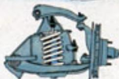
□ Radial-tuned suspension package helps improve ride and handling with Camaro's standard radial ply tires. Includes larger front and added rear stabilizer bars plus special front and rear shock absorbers.
