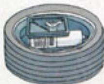
□ Space-Saver tire takes up less trunk room than regular spare. Comes with compressed gas canister for inflation.
