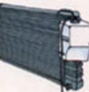
Coolant recovery system helps prevent coolant loss and overheating.
