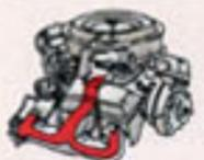
\*Early Fuel Evaporation system speeds up engine warm-up by using exhaust gases to heat incoming fuel-air mixture.
