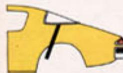
Steel cargo-guard divides trunk from passenger compartment to help keep what's in the trunk in the trunk.
