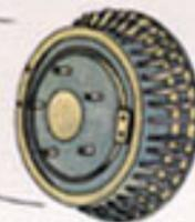
New finned rear brake drums run cooler, resist fade.
