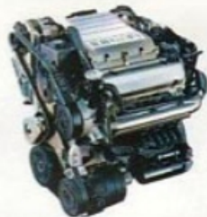
The 125-horsepower 2.8 liter V6, now with direct-fire ignition, standard in Cimarron.
