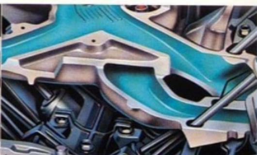
Dual-level intake system for improved engine response.
