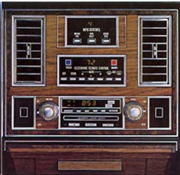
MPG Sentinel shows number of active cylinders. (With V8-6-4 engine only.)
