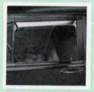
VENTSHADES—Functional stainless steel window shields not only dress up the car but, in addition, perform many useful duties. They cut annoying sun glare... reduce drafts from open windows... permit lowering windows two or three inches during a rain storm without letting rain in.
