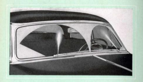
WINDSHIELD WASHER—Once considered a convenience item, the Cadillac windshield washer has rapidly come to be accepted by owners as a safety must. It sprays two jets of water and solvent mixture on the windshield so that mud, slush, road spray or insects can be easily swept away by the windshield wipers. A touch of the button in the center of the wiper switch gives immediate action.
