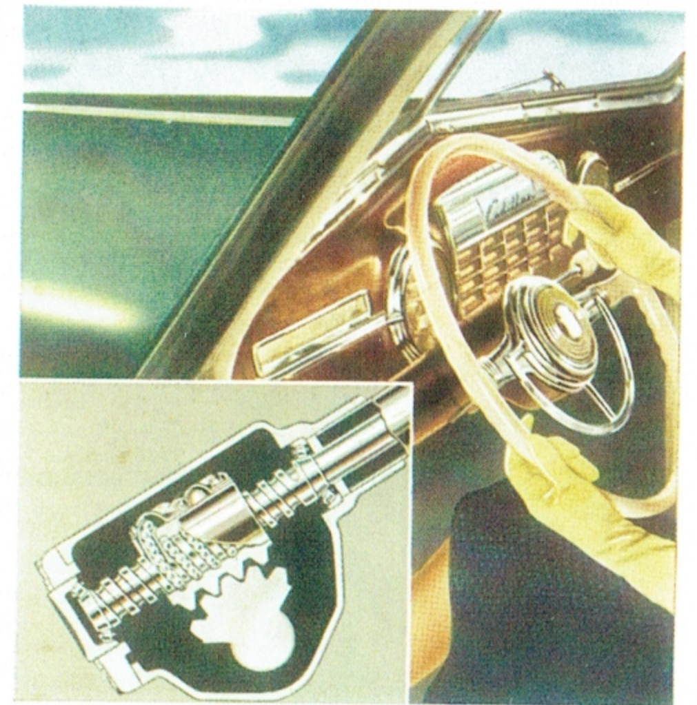
The ball bearing steering gear was pioneered by Cadillac. This important new advancement, shown in inset, is not only stronger than conventional assemblies, it also gives Cadillac cars unexcelled steering ease.
