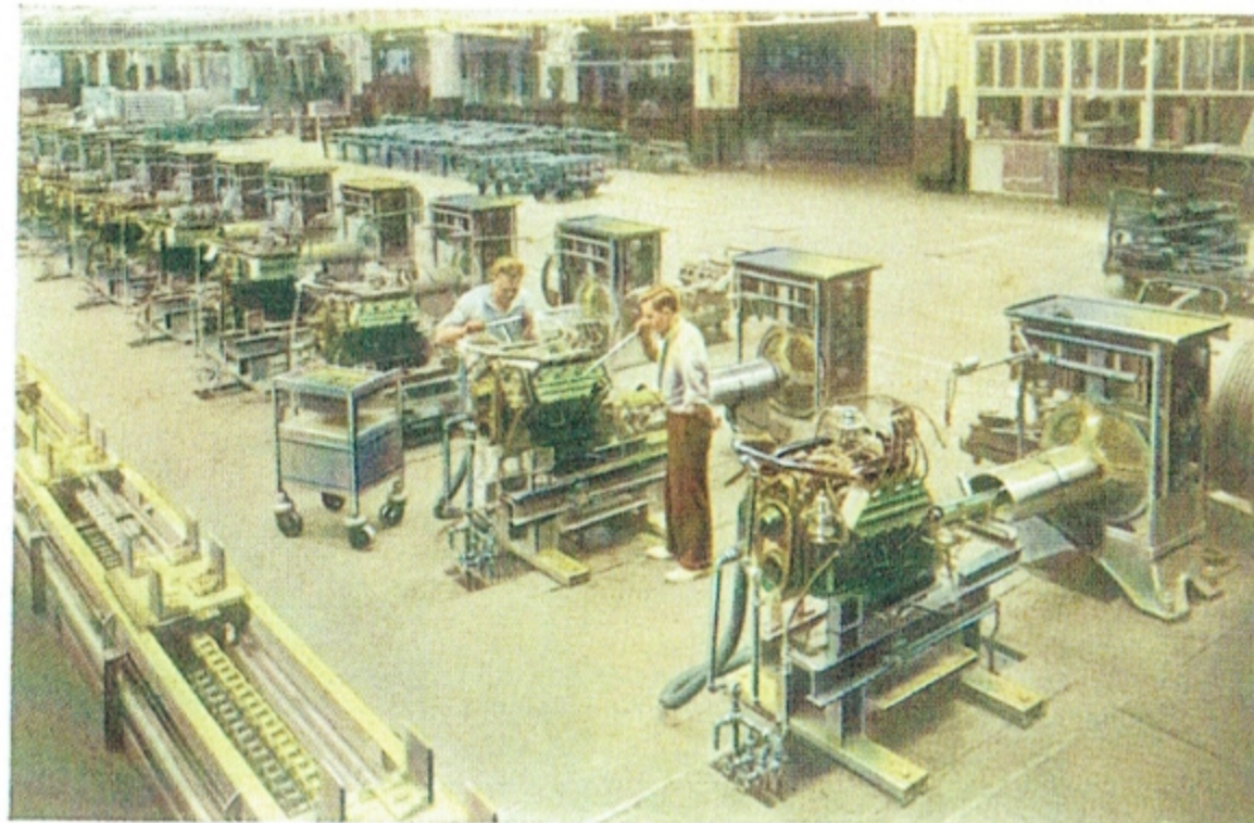
The block test given to every Cadillac engine serves a double purpose. Engines are run continuously for many hours, thereby thoroughly breaking them in. Meanwhile, smoothness, quietness, and compression are checked and rechecked by accurate machines.
