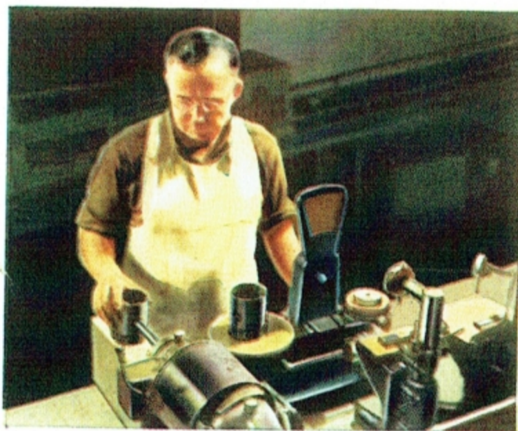
In a special room kept constantly at 72 degrees F., every Cadillac piston is weighed and graded to afford a selective bore fitting within 7/100,000 inches maximum variation—about 1/40 the width of human hair. Wrist pin holes are "bearingized" to a four-millionth inch surface finish.
