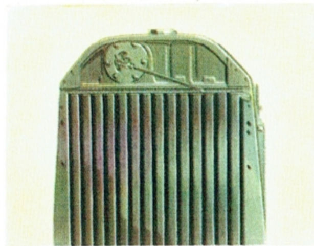
Automatic radiator shutters maintain higher winter underhood temperatures. Gas vaporizes better and sludge formation is checked.
