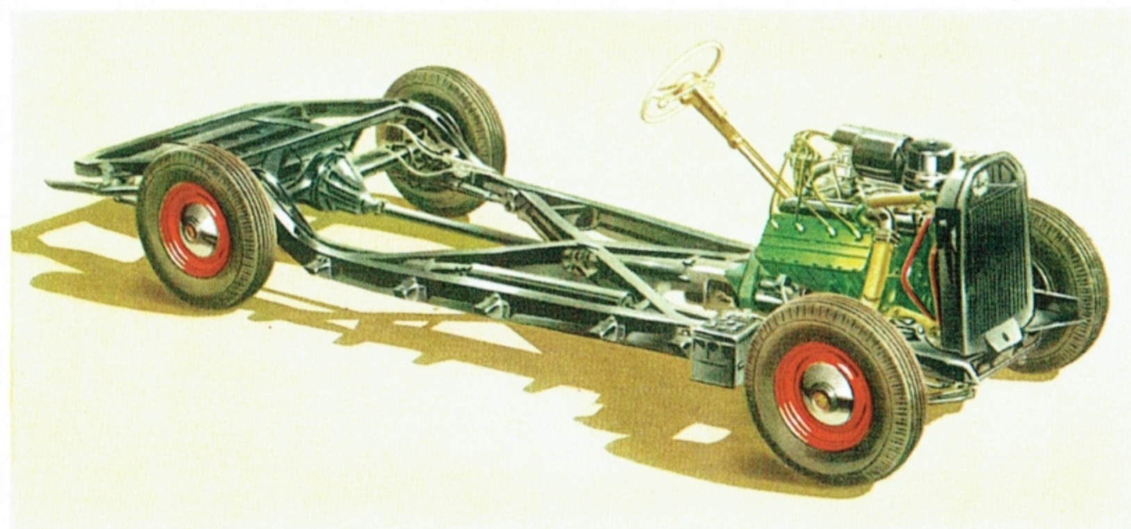
As this massive chassis shows, Cadillacs are built to run better for a longer time at less upkeep cost than other cars. The new frame is 40% stronger. Brakes, clutch, and other
