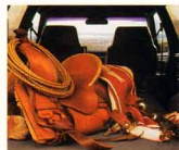
The rear bench seat folds down to provide a cargo area 76 inches long and a capacity of more than 74 cubic feet.
