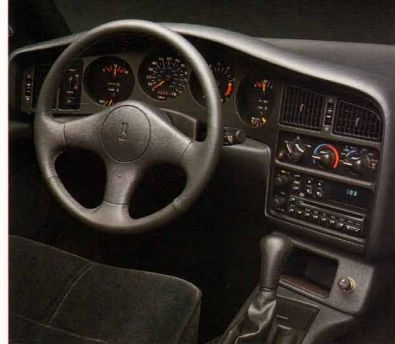
Left: The wraparound dash features full analog instrumentation. The steering column stalk controls include a one-step "flash-to-pass" feature and a wiper/washer switch that activates a washer built into the wiper arm itself to help avoid freeze-up.
