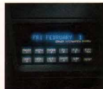
THE AVAILABLE DRIVER INFORMATION SYSTEM GIVES DIGITAL READOUT OF FUEL ECONOMY, AMOUNT OF FUEL USED, ESTIMATED ARRIVAL TIME, ESTIMATED OIL LIFE, AVERAGE SERVICE REMINDERS, ETC. (AVAILABLE 11/90.)
