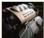
THE STANDARD 3800 V6 ENGINE WITH TUNED PORT INJECTION PROVIDES 170 HORSEPOWER.
