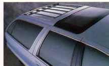
THE VISTA ROOF IS MADE OF SOLARCOOL GLASS TO REDUCE THE SUNLOAD, AND FLOWS SMOOTHLY INTO THE INTEGRATED ADJUSTABLE LUGGAGE RACK.
