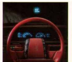
THE AVAILABLE HEAD-UP DISPLAY ON THE INTERNATIONAL SERIES PROJECTS THE VEHICLES SPEED ONTO THE WINDSHIELD, FREEING THE DRIVER FROM CUTLASS SUPREME LOOKING DOWN AT THE SPEEDOMETER.
