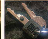
THE PASS KEY THEFT DETERRENT SYSTEM DISCOURAGES THEFT WITH AN ELECTRONICALLY ENCODED KEY.
