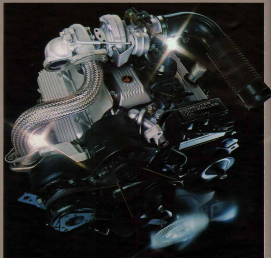
Regal 3.8 litre SFI turbocharged engine.
