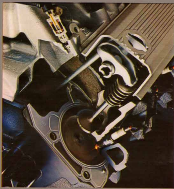
3.8 litre engine cutaway with injector.
