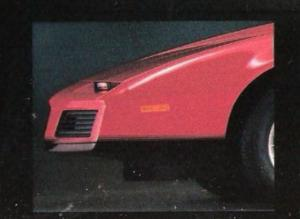
Front air dam directs air around the body, keeping lift forces to a minimum.
