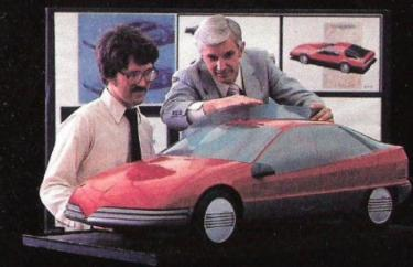
Then the full-size clay model is shaped by conventional methods on a rigid steel armature to which, if necessary,
