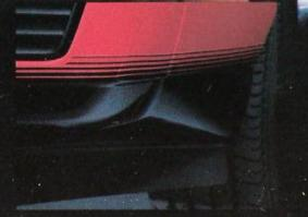
Front and rear wheel skirts channel air away from the wheel housings to keep it flush with the body.
