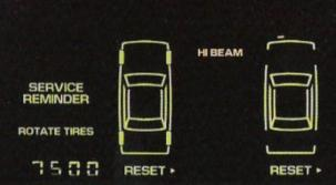
The Driver Information Center is a liquid crystal graphic display that tells you when the temperature is high, when the fuel, oil, coolant and washer fluid is low, when the hood or trunk is open, and when and which door is ajar. The Driver Information Center also allows you to check your headlights, hi-beams, turn signals, brakes and taillights, all from the driver's seat. It even
