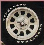
□ Steel-belted, radial-ply white billboard lettered BR70-13 tires supplied by various manufacturers*
