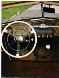
Wood-grained trim is nothing new to Buick. This 1938 Buick Special featured a dashboard which looked for all the world as though it were carved from a solid block of walnut. (In reality, it was metal.) Other interior refinements included a 270°-sweep speedometer, surrounded by a complete set of gauges. The steering wheel and gearshift knob were done in striking mother-of-pearl.
