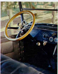
In 1922, this 4-cylinder Buick Touring Car represented the very latest in comfort and convenience. The quadrant, in the center of the polished wood steering wheel, controlled spark advance; while separate gauges monitored engine oil pressure and amperes. The windshield was hinged at the center, so fresh air could be directed to the occupants.
