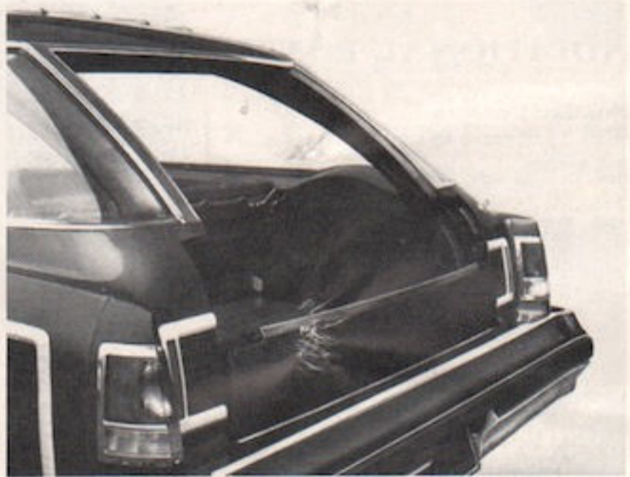
Power Operated Tailgate (Code 522—UPC C26). Pontiac's "disappearing tailgate" slips under the floor and out of the way. Available on Catalina Safari and Grand Safari. (Power operated tailgate window is standard with this option.) (F)
