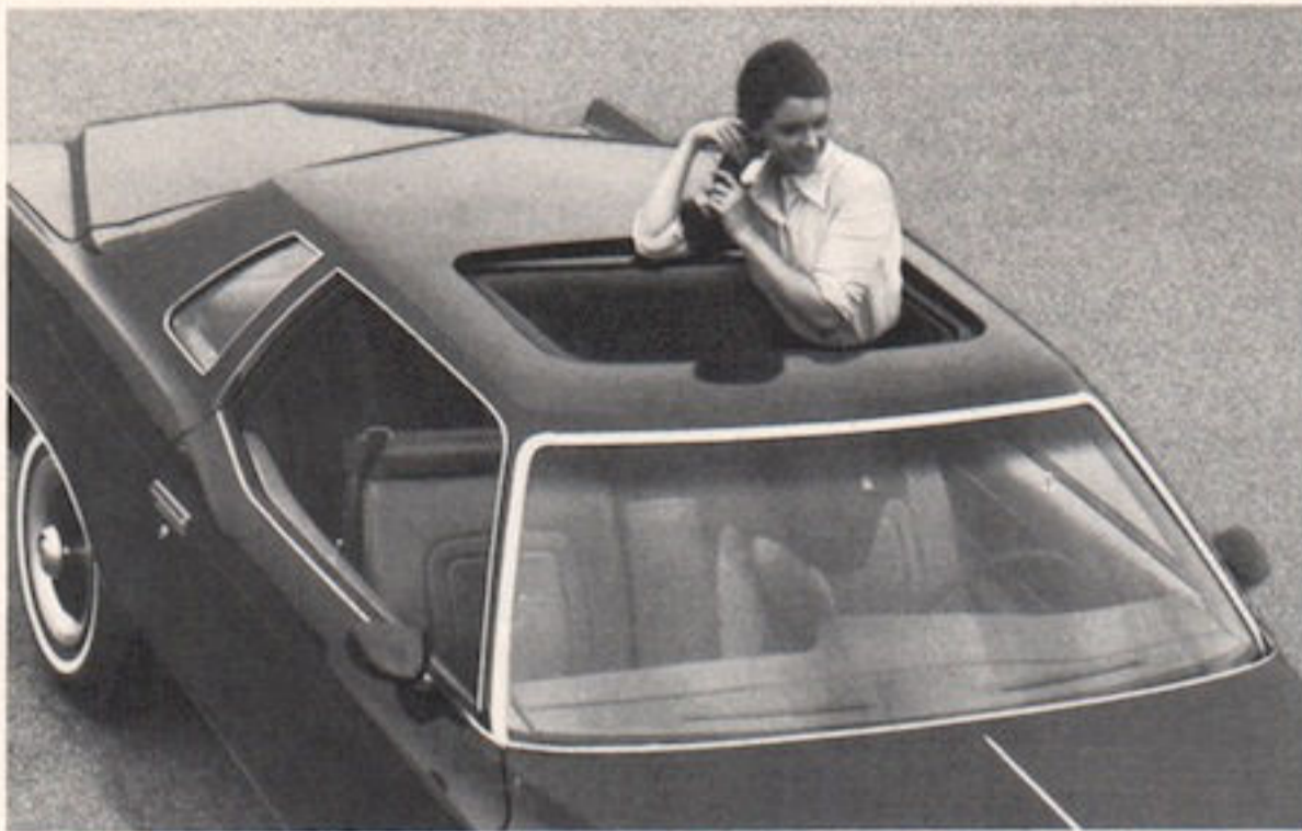
Metal Sliding Sunroofs (Code 452—UPC CA1 power operated; Code 454—UPC CO3 manual). Available on 2-door models only, LeMans, LeMans Sport Coupe, Luxury LeMans, Grand Am and Grand Prix. (F)
