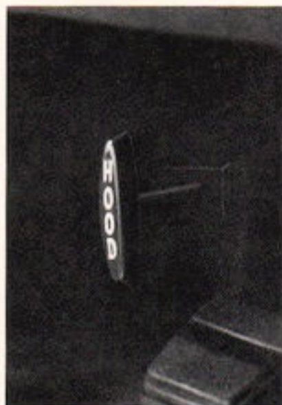
Inside Hood Release. Unlocks hood from inside car only; protects against engine component thefts. Available on Firebird models; standard on all other models except Pontiac Ventura and Ventura Custom. (D)
