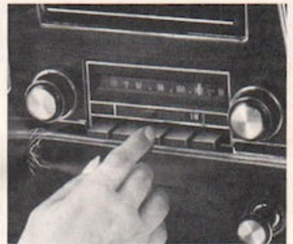
AM/FM Radio (Code 413—UPC U69). Completely transistorized. Available on all models. (F,D)
