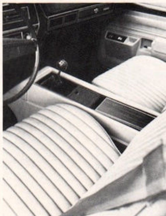
Console for LeMans Sport Coupe and Luxury LeMans with Manual Transmission (Code 431-UPC D55). Available with three- or four-speed manual transmission with bucket seats on LeMans Sport Coupe, and on the Luxury LeMans 2-dr. models with bucket seats. Console features a soft, padded-vinyl exterior covering, color-keyed to match interior. (F)
