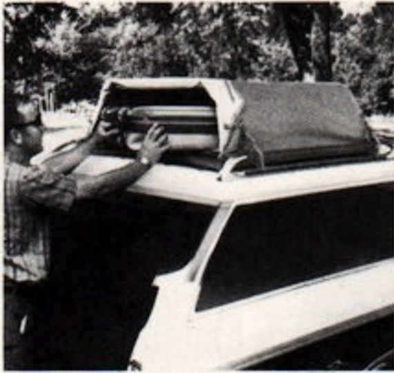
Luggage Carrier Cover—Rakpak. Heavy-duty treated fabric protects luggage from water and dust. Off the car, cover folds flat for convenient storage. Ties down neatly into top of Chrome Luggage Carrier. Version for Catalina Safari and Grand Safari (size—40" x 42" x 14") opens from the rear. LeMans Safari version (size—36" x 48" x 14") opens from the side. (D)
