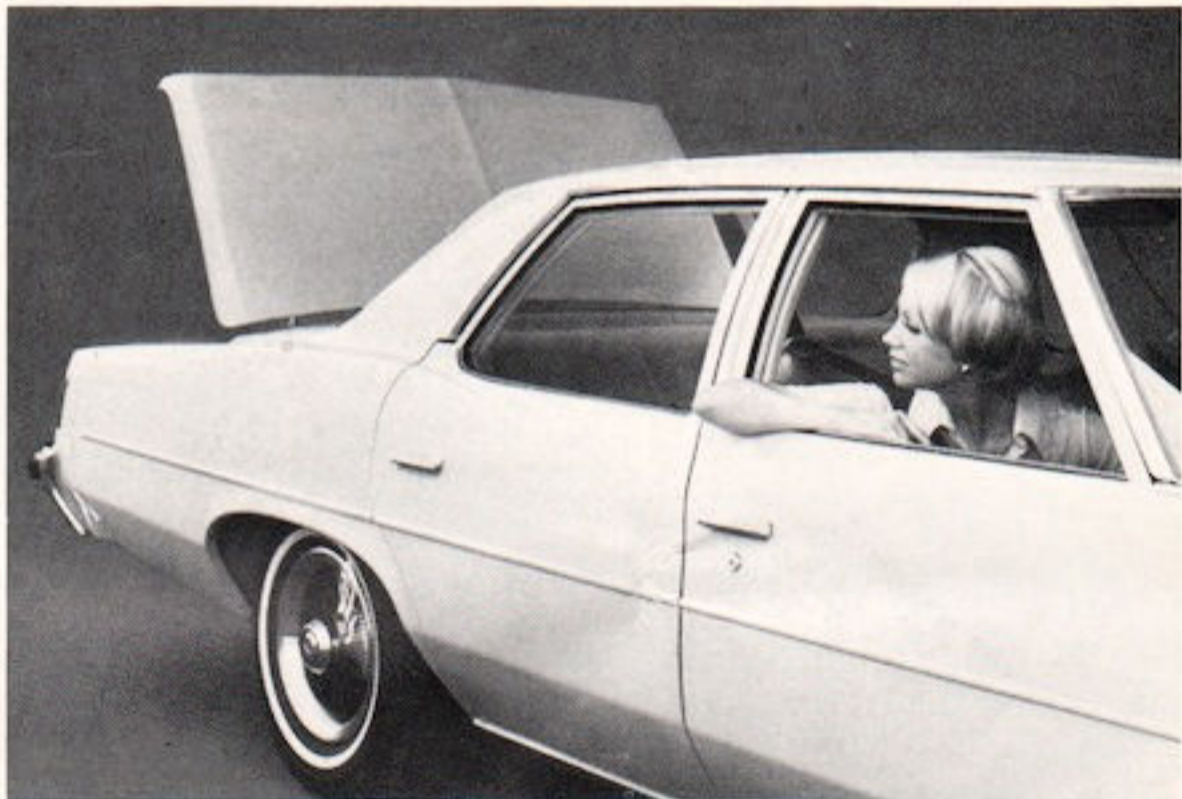
Deck-lid Release (Code 694—UPC A90). Just press button inside glove box or console to unlock the trunk. Trunk also can be closed and opened in the conventional manner. Available on all models except station wagons, Ventura and Ventura Custom. Dealer installed only on Firebird models. (F,D)
