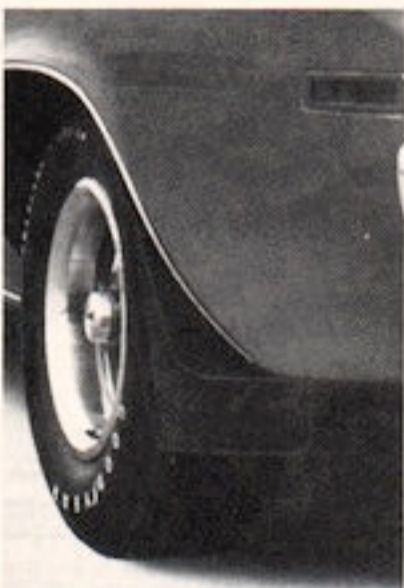
Fender Splash Guards. Protect rocker panels from dirt and stone nicks; adds sporty look. Available all models, front and/or rear. (D)
