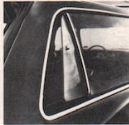
Swing-out Glass Rear Quarter Vent (Code 521—UPC A20). Standard on three-seat LeMans Safari and Luxury LeMans Safari; available on two-seat LeMans Safari and Luxury LeMans Safari. (F)
