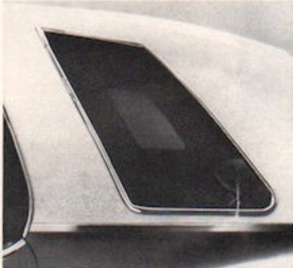
Formal Roof Option (Code 341—UPC WY2). Standard on Grand Prix. Standard on Luxury LeMans Colonnade Hardtop Coupe (only with Landau or Cordova Top until early 1974). Available on LeMans Sport Coupe with Landau or Cordova Top. (F)
