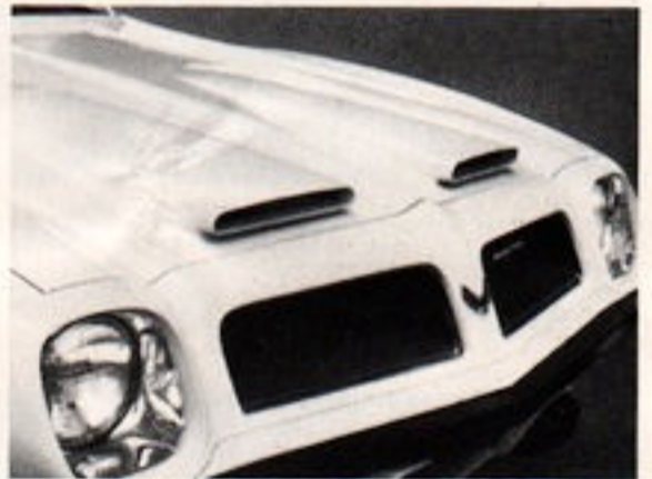
Ram Air Hood (Code 514—UPC WU3). Only on the Firebird Formula. Available with 400-cu.-in. and 455-cu.-in., 4-bbl. V-8 engines. (F)
