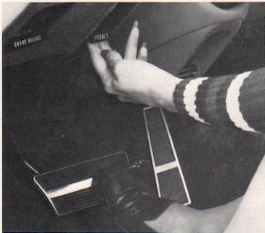
Adjustable Pedals (Code 502—UPC WX7). Allows brake and accelerator to be positioned so driver can reach them without moving seat to a position otherwise uncomfortable for him. Adjustment lever is located left of steering column. Available on Catalina, Bonneville, Grand Ville, Catalina Safari and Grand Safari. Pedal trim standard with adjustable pedal on all models. (F)
