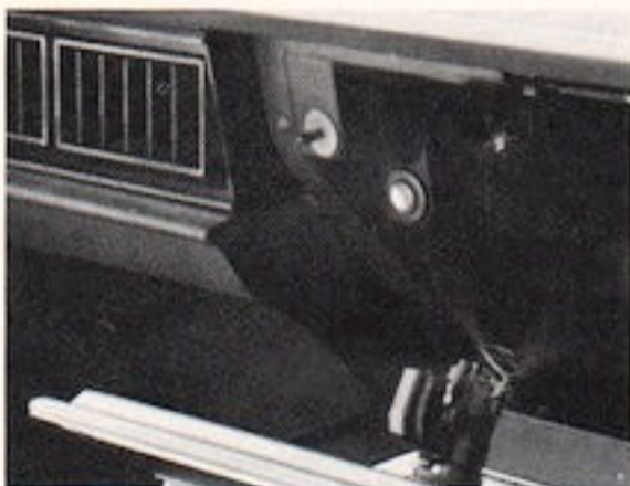
Deck-lid Release (Code 694—UPC A90). Just press button inside glove box or console to unlock the trunk. Trunk also can be closed and opened in the conventional manner. Available on all models except station wagons, Ventura and Ventura Custom. Dealer installed only on Firebird models. (F,D)
