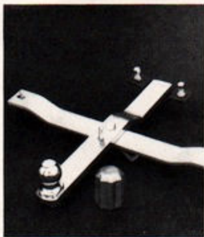
Trailer Hitch (Code 701—UPC VR2). A Class I hitch to be used in towing light trailers (up to 2,000 pounds loaded) with light tongue loads (up to 200 pounds). Chrome-plated draw bar and 1 3/4" diameter ball. Permanently bolts to structural members of the car. Available in custom designs for every Pontiac model except Ventura and Ventura Custom, Firebird, Firebird Esprit, Firebird Formula and Firebird Trans Am (F.D). Another hitch is available for these models to be used in towing very light trailers (up to 1,000 pounds gross weight and 100 pounds tongue load). (D)
