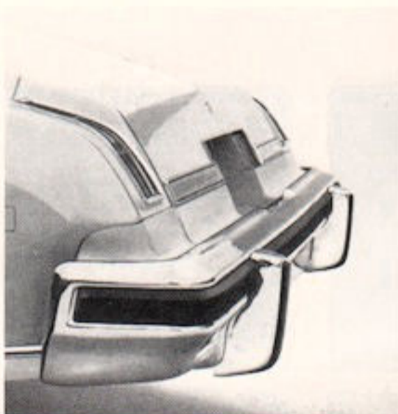
Rear Bumper Guards (Code 732-UPC V32). Chrome with rubber facing strip. Available on LeMans, LeMans Sport Coupe, Luxury LeMans, Catalina, Catalina Safari, Bonneville, Grand Ville, Grand Safari and Grand Prix. (F,D)
