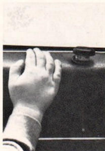
Child Guard Door Locks. Prevent children from opening rear doors. Can be unlocked only with ignition key. Available on all four-door models. (D)
