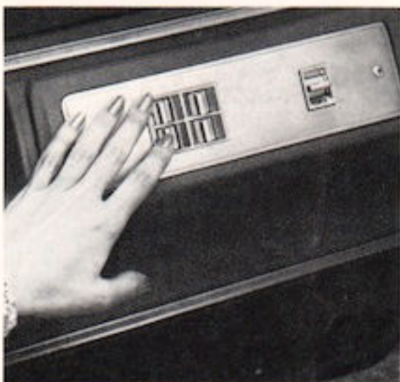
Power Windows (Code 551—UPC A31). Individual passenger switches and a central panel on driver's door (console on Firebird, Firebird Esprit, Firebird Formula and Firebird Trans Am). Windows will not operate when ignition is off. Available on all models except Ventura and Ventura Custom. Available on Firebird models, with console only. (F)
