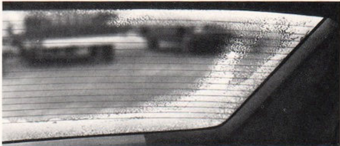
Electrically-heated Rear Window Defroster (Code 592—UPC C49). Includes Soft-Ray glass in rear window. Available on all models except Ventura and Ventura Custom and Grand Ville Convertible. (F)
