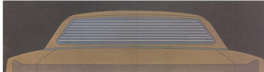
Been wondering where we hid the radio antenna? The diagram (top) shows it. Two .005" wires are embedded in the middle of the windshield. The radio at the other end can be AM, AM/FM or AM/FM with FM stereo multiplex. Specify your choice.
