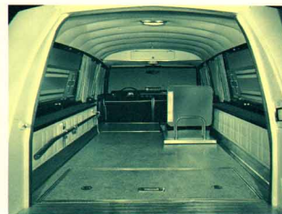
FOR AMBULANCE SERVICE: Table is removed, attendant seat unfolded from stepwell, cot fastener inserted, and insignia placed in windows. Stretcher compartment in floor, extra.
