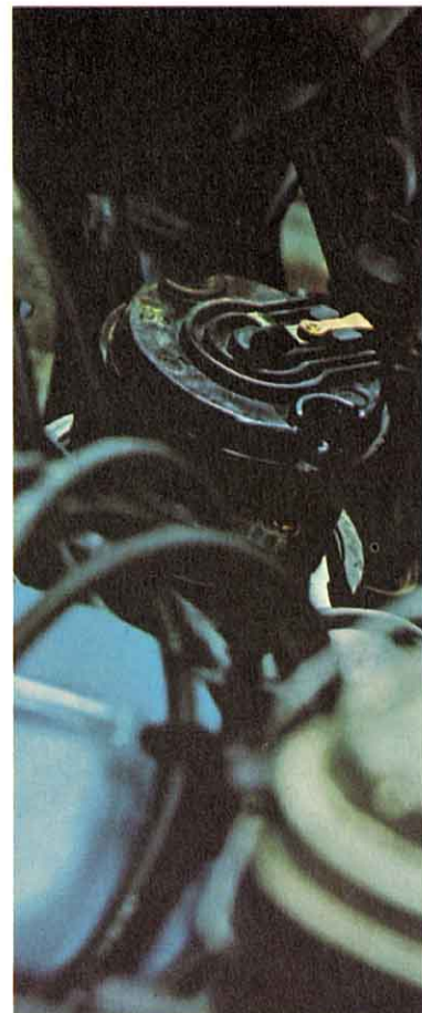
Delco transistorized ignition. No points, no condenser. Next best thing to a magneto. Extra cost.
