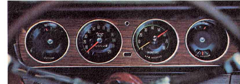
New instrumentation. Fuel and ammeter; 250° tach where it should be—beside speedo; water temp, oil pressure gauges. Extra cost.
