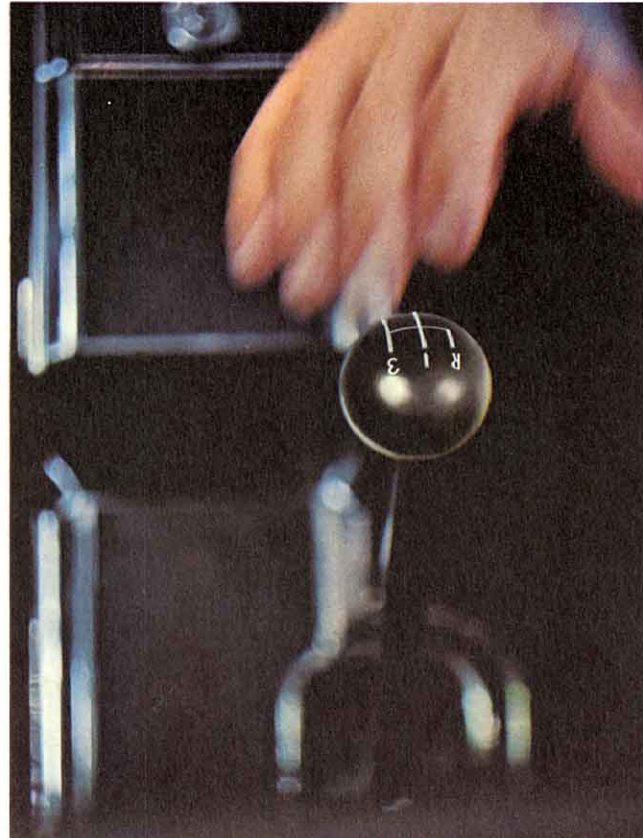
The 4-speed comes with a close-ratio gear set and Hurst floor shift. Extra cost, as is the optional console.
