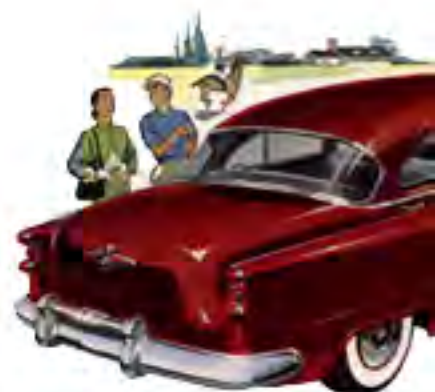
A sleeker look and more storage space are the results of raising the rear fenders and the deck profile. The 1953 Special looks bigger because it is bigger. The trunk compartment capacity has been increased 537 cubic inches.
