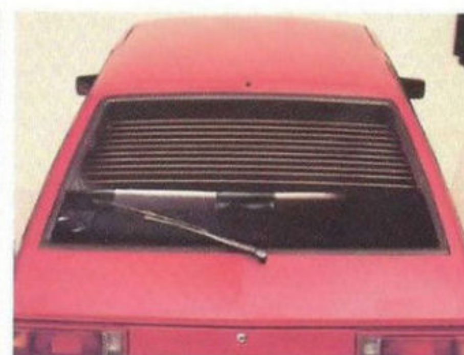
Rear Window Defroster and Washer/Wiper. The defroster is optional on base models only; the washer/wiper system is optional on all Champs except LS.
