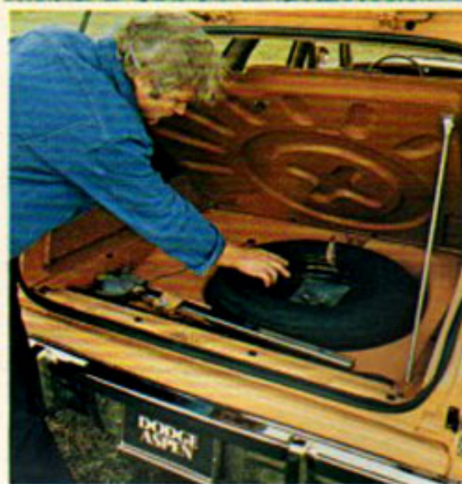
Concealed tire stowage for unobstructed load floor.
