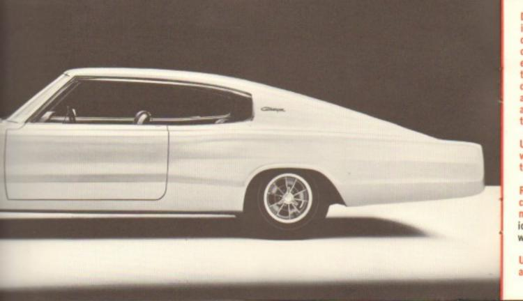
Developed to demonstrate advanced ideas, Charger II is a styling show car which presents fresh, new directions in design from Dodge. From a Delta-ornamented hood to its fastback rear deck, the emphasis is on clean, sweeping lines. Nothing protrudes. A concealed latch eliminates conventional door handles. Charger II needs no vent panes. Fresh air enters three large cowl intakes in controlled amounts. It circulates gently and quietly through the interior, flows out vents atop each rear fender.
