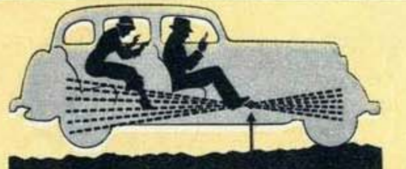
THE OLD WAY. Stiff front springs and 60 per cent of weight on rear springs gave a "bouncy" ride.
