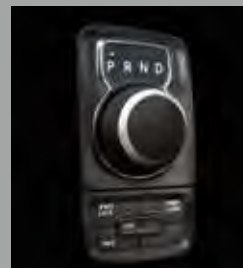
Mated to the Pentastar V6 is the new TorqueFlite 8-speed — fully electronic, and featuring an all-new Rotary Shifter.
