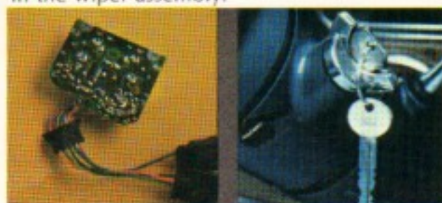
Solid-state ignition doesn't require breaker point replacement
