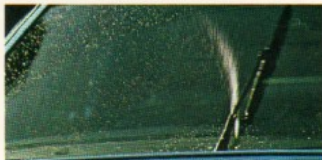
Windshield washer jets are mounted in the wiper assembly.
