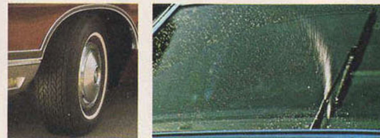
Steel-belted radial ply tires are standard on every Mercury series for 1975; windshield washer jets are concealed in the wiper assembly.
