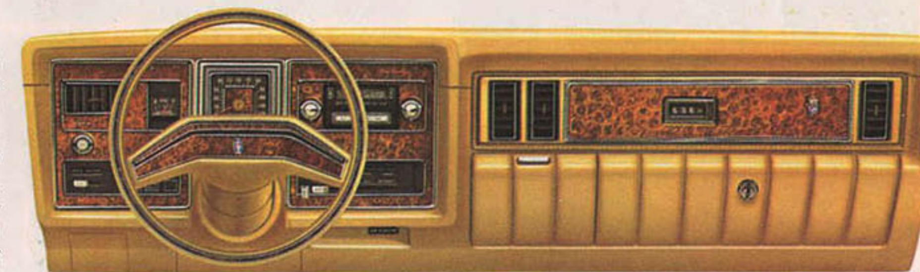
Mercury Monarch Ghia instrument panel with optional AM/FM/Multiplex stereo radio and tape player.
