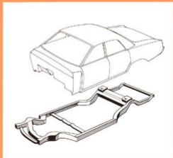
Two-Piece Body-and-Frame Construction used by most competitors. Separate frame is bolted to underside of car body.
