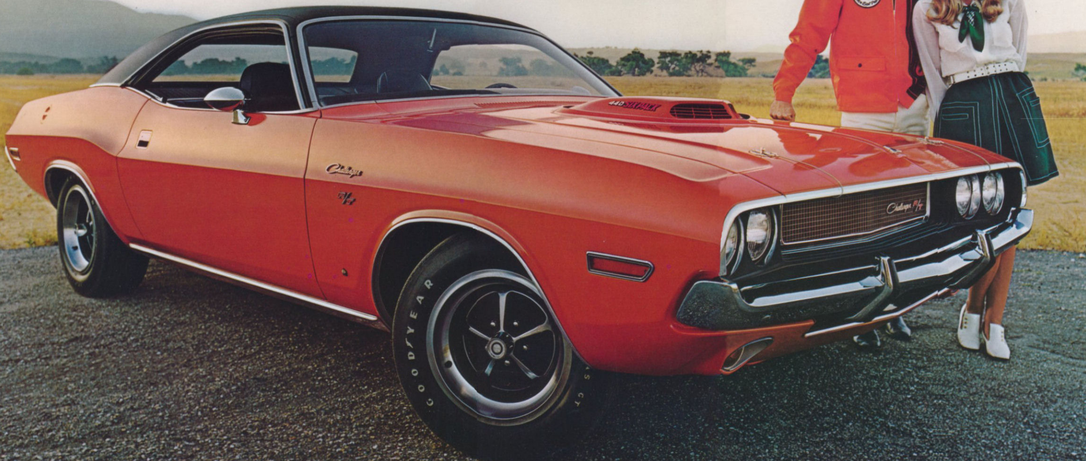
"Shaker" hood? Yes, functional scoop attached directly to carbs "shakes" at idle.
